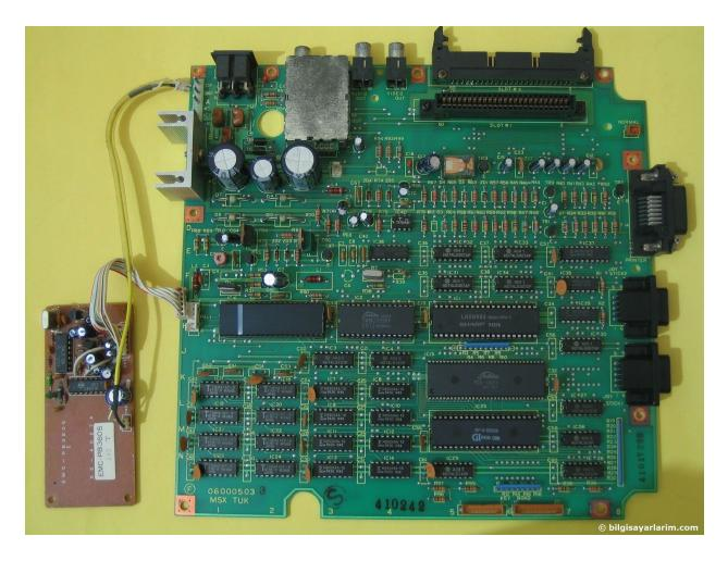
On some computers like the HX10 the **SOUNDIN** (pin 49) seems not connected. You can fix that, find the audio combine inout point of the audio amplifier on the PCB by following the resistor/capacitor line from the cartridge connector to pin 49 on the cartridge slot. A bit complicated without circuit diagram to explain, it is usually a resistor and a capacitor in series. Here is how GDX did it on a HX-10.
