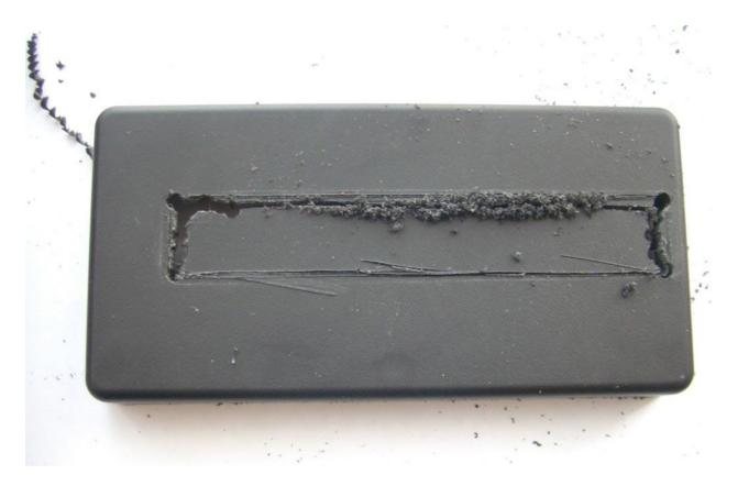
7) The slot for the cable is easily inserted with the flat file.
