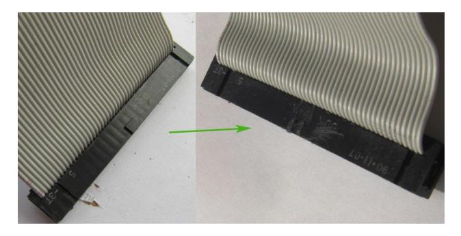
4) Separate each wire on the other end about 1 cm with a cutter and cut all even cables (2, 4, 6,  $\sim$ , 50) 6 mm with scissors.
