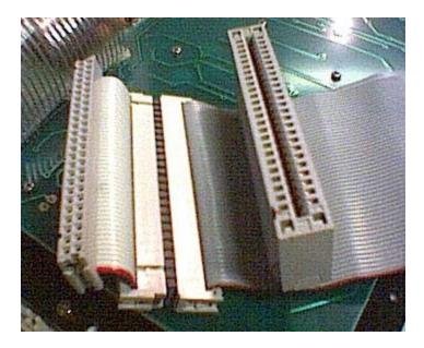
If the cartridge connector is the PCB type, you might use an experimenters print and solder the wires.
