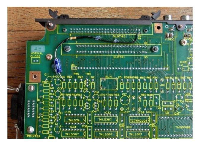
Pin 49 of the SLOT-3 is connected to a 10 K $\Omega$  resistor which is connected to the (-) side of a 10  $\mu$ F capacitor. The (+) side goes to the amplifier. Now the Slot is 100% functional.
